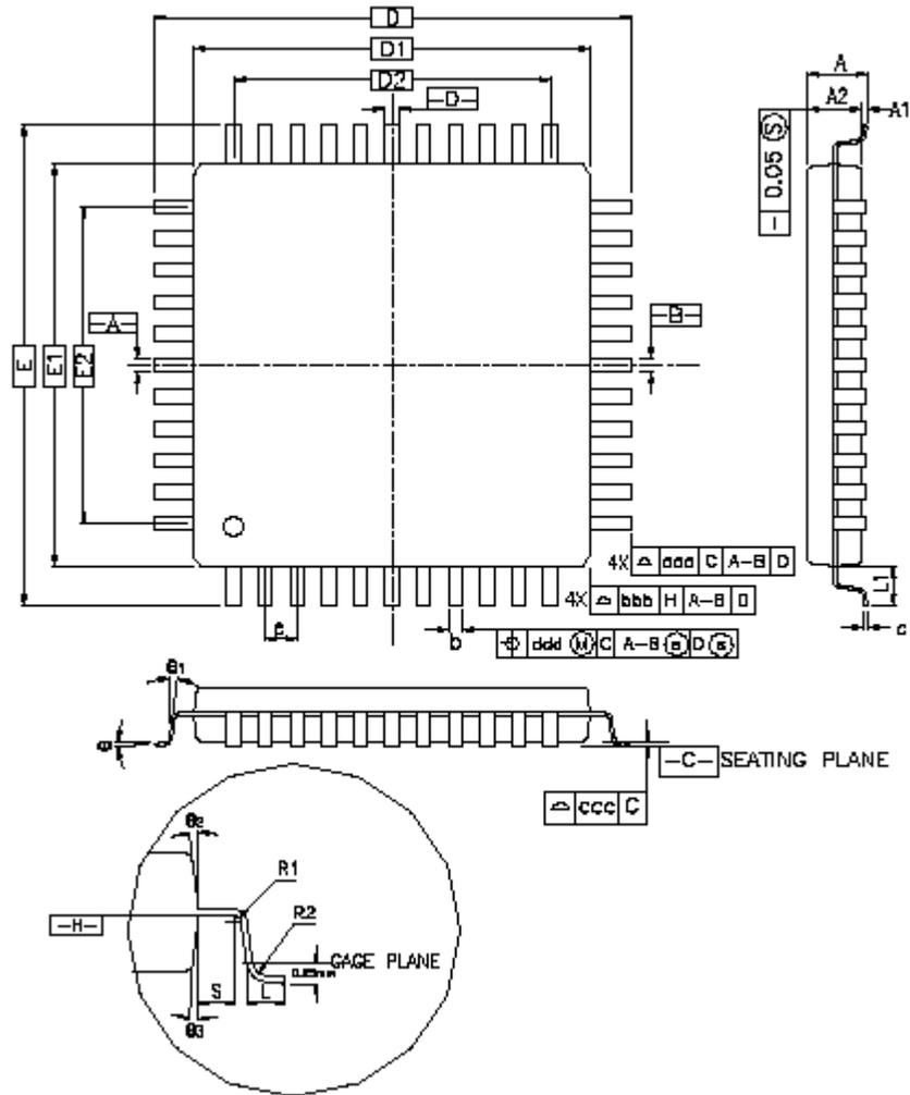
**Table 38-1.** 48-lead LQFP Package Dimensions (in mm)
