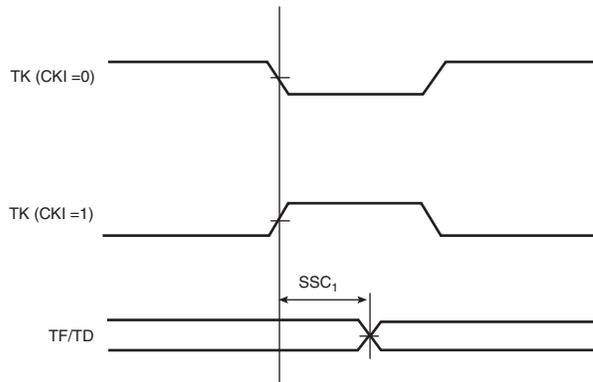
**Figure 37-10.** SSC Transmitter, TK in output and TF in input
