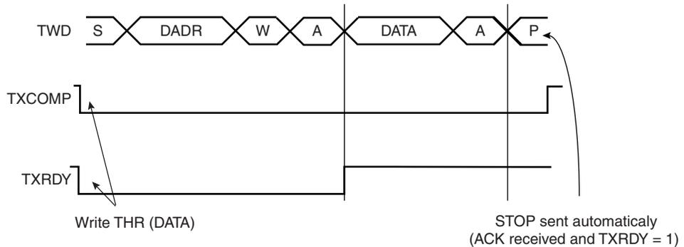
**Figure 30-7. Master Write with Multiple Data Byte**
