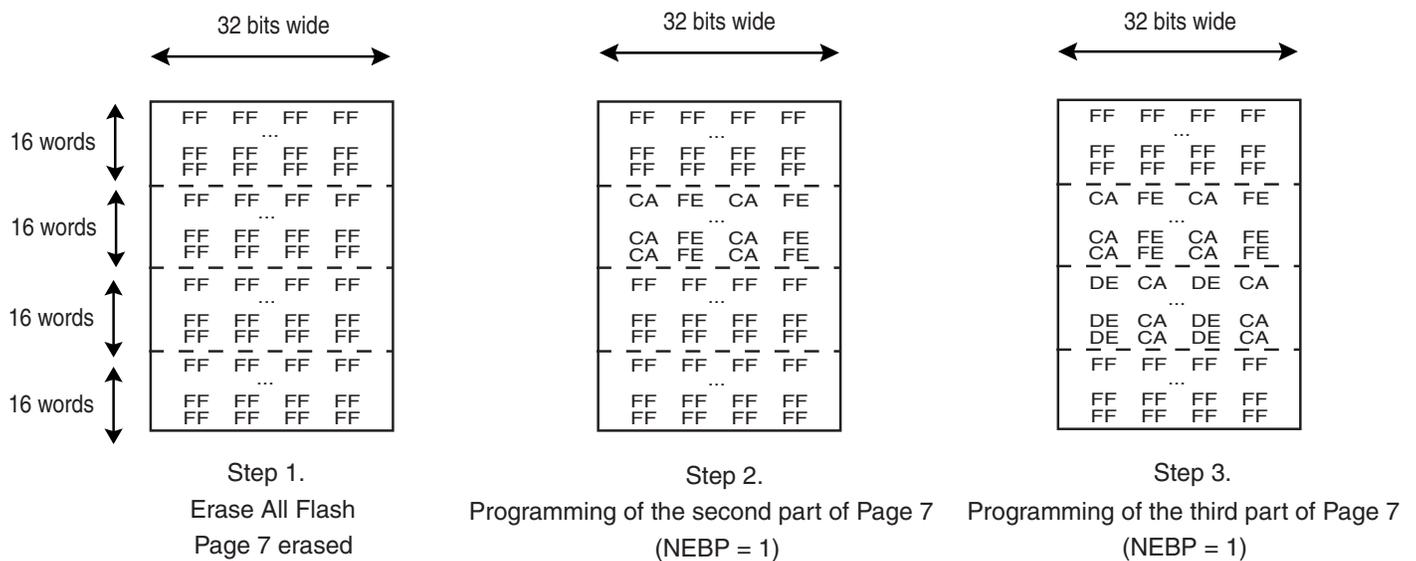
The Partial Programming mode works only with 32-bit (or higher) boundaries. It cannot be used with boundaries lower than 32 bits (8 or 16-bit for example).
