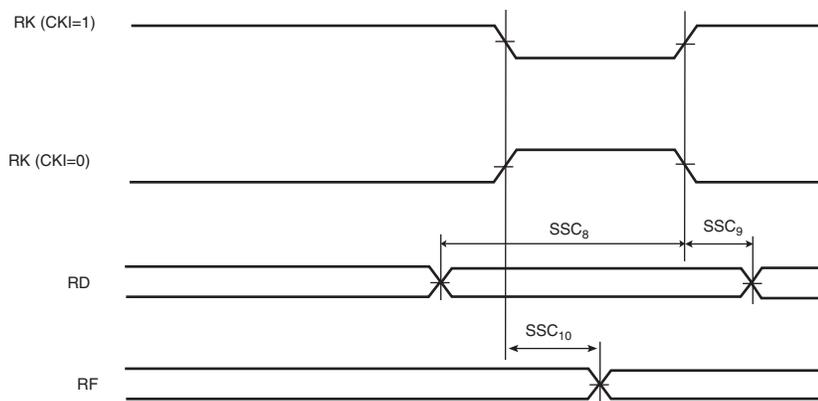
**Figure 37-14. SSC Receiver, RK and RF in output**
