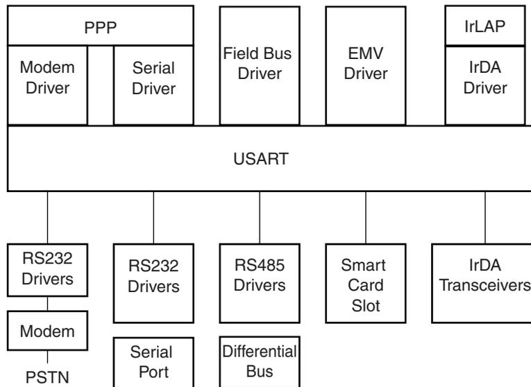
**Figure 31-4.** AT91SAM7S32/16 Application Block Diagram
