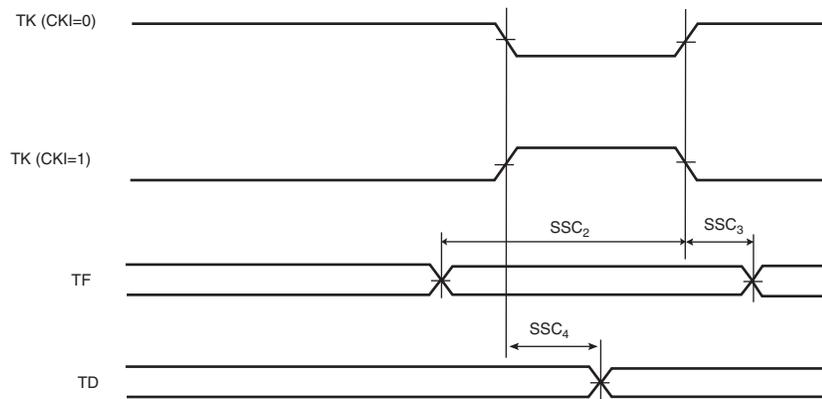
**Figure 37-11. SSC Transmitter, TK and TF in input**
