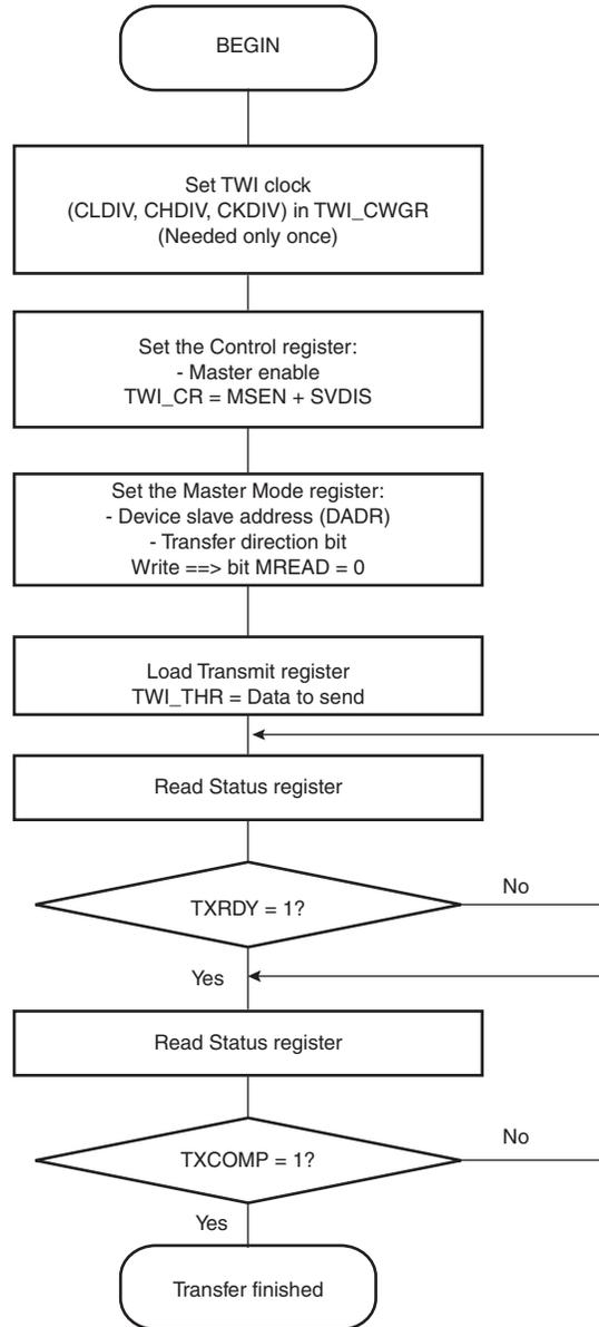
**Figure 30-15.** TWI Write Operation with Single Data Byte and Internal Address
