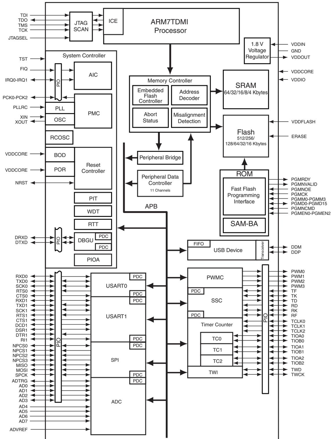
Figure 2-2. AT91SAM7S32/16 Block Diagram
