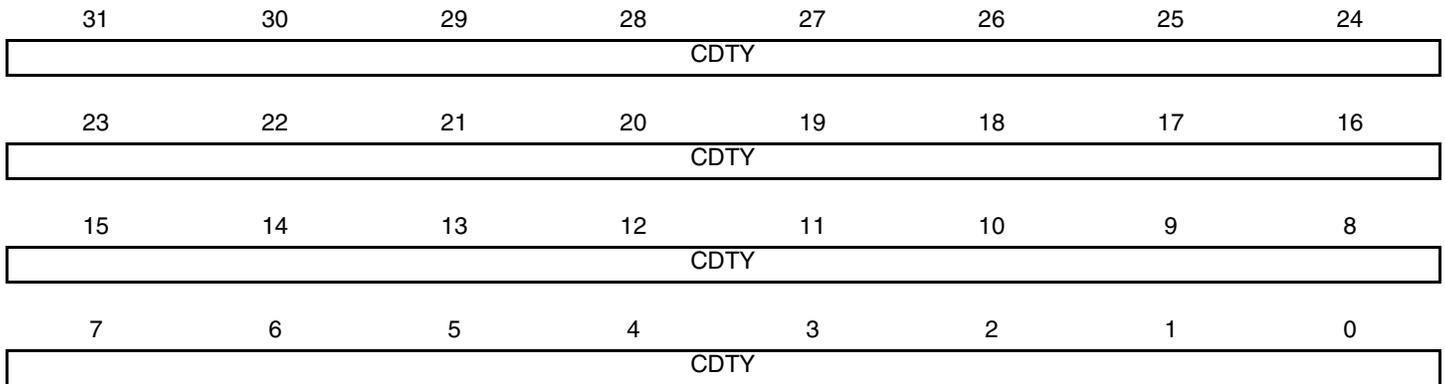
Only the first 16 bits (internal channel counter size) are significant.
