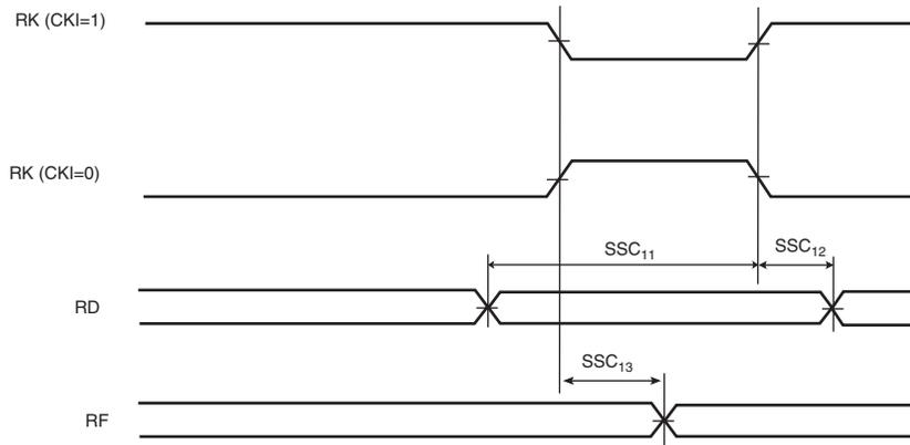
**Figure 37-15. SSC Receiver, RK in output and RF in input**
