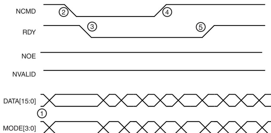
**Figure 20-4.** AT91SAM7S32/16 Parallel Programming Timing, Write Sequence
