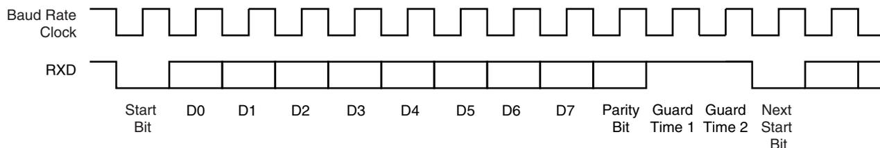
**Figure 31-24.** T = 0 Protocol with Parity Error
