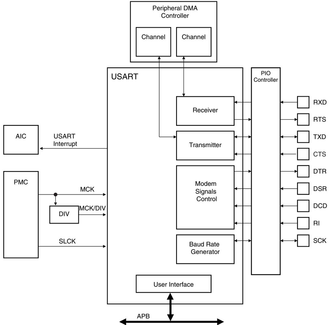
**Figure 31-2.** AT91SAM7S32/16 USART Block Diagram
