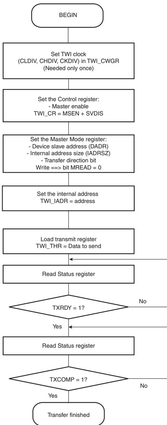
**Figure 30-16.** TWI Write Operation with Multiple Data Bytes with or without Internal Address
