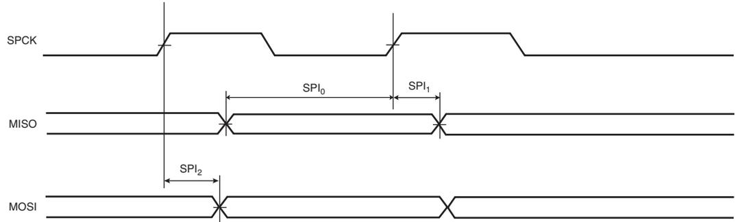
**Figure 37-5.** SPI Master mode with (CPOL=0 and NCPHA=1) or (CPOL=1 and NCPHA=0)
