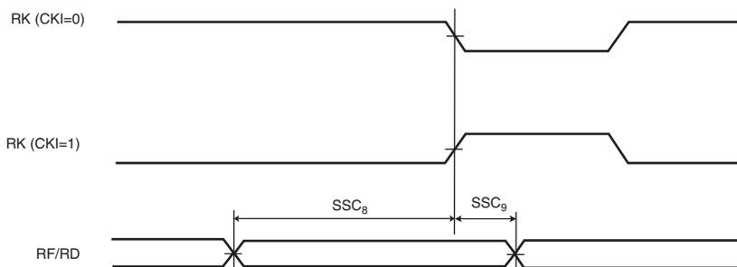
**Figure 37-13. SSC Receiver, RK in input and RF in output**
