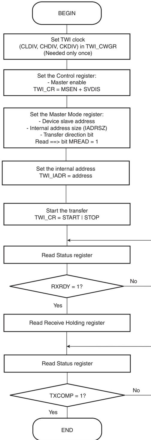
**Figure 30-19.** TWI Read Operation with Multiple Data Bytes with or without Internal Address
