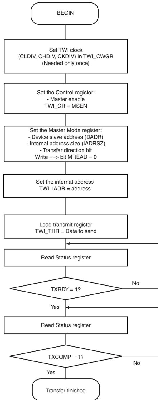
**Figure 29-15.** TWI Write Operation with Multiple Data Bytes with or without Internal Address
