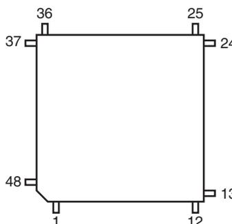
**Figure 4-4.** 48-pad QFN Package (Top View)
