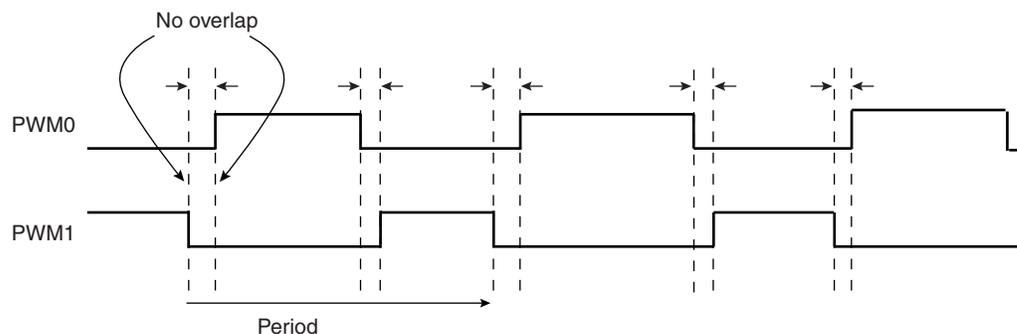
Note: See [Figure 34-5 on page 483](#) for a detailed description of center aligned waveforms.
