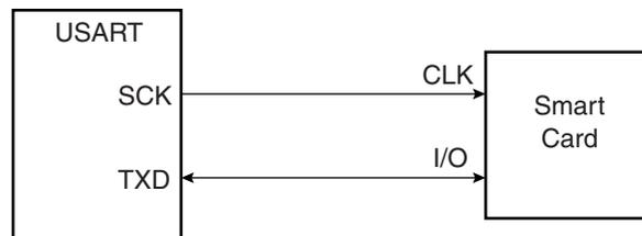
When operating in ISO7816, either in T = 0 or T = 1 modes, the character format is fixed. The configuration is 8 data bits, even parity and 1 or 2 stop bits, regardless of the values programmed in the CHRL, MODE9, PAR and CHMODE fields. MSBF can be used to transmit LSB or MSB first. Parity Bit (PAR) can be used to transmit in normal or inverse mode. Refer to [“USART Mode Register” on page 388](#) and [“PAR: Parity Type” on page 389](#).
