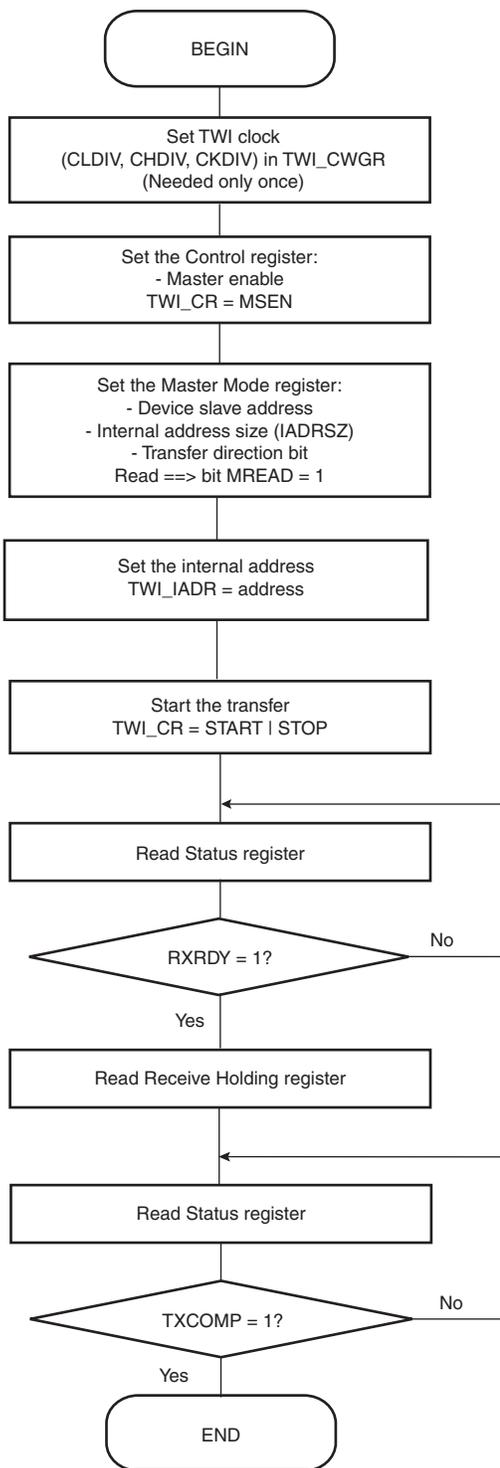
**Figure 29-18. TWI Read Operation with Multiple Data Bytes with or without Internal Address**
