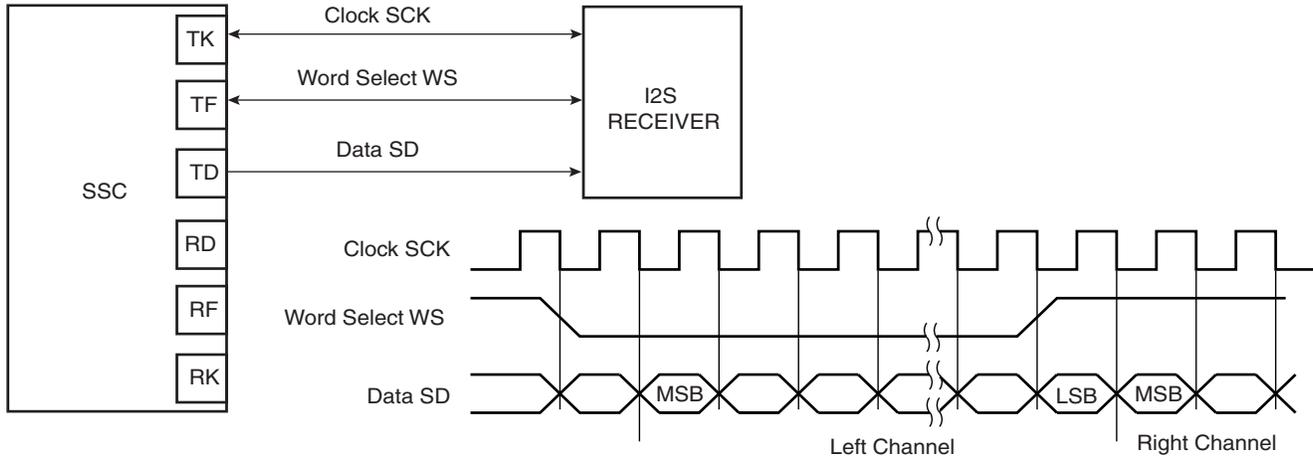
**Figure 32-18.** Codec Application Block Diagram
