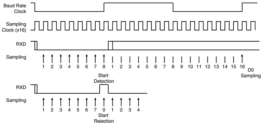
**Figure 31-11. Asynchronous Character Reception**
