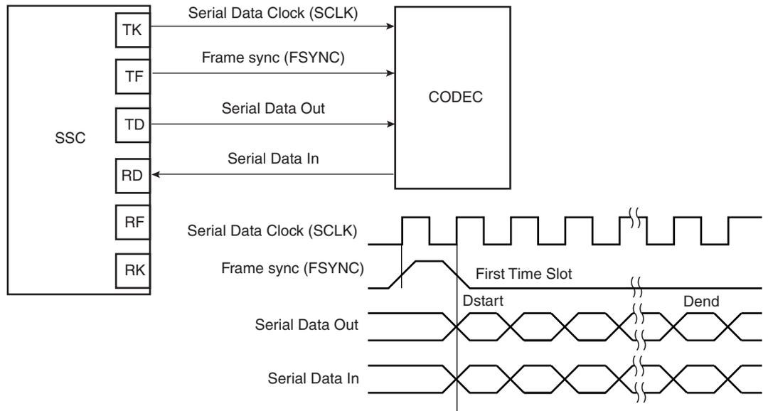
**Figure 32-19.** Time Slot Application Block Diagram
