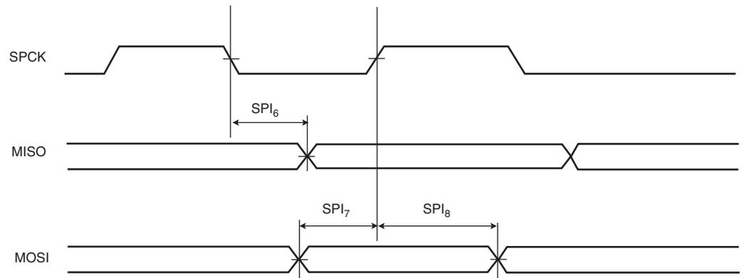
**Figure 37-7.** SPI Slave mode with (CPOL = NCPHA = 0) or (CPOL= NCPHA= 1)
