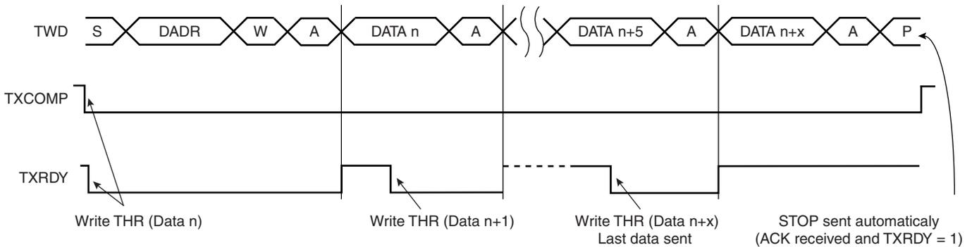
**Figure 30-8. Master Write with One Byte Internal Address and Multiple Data Bytes**
