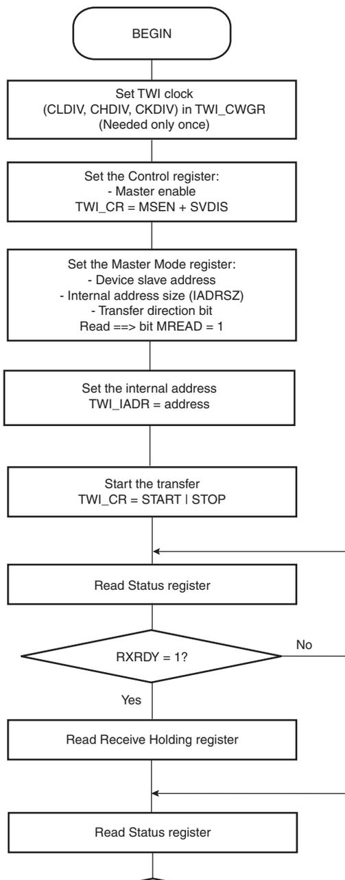
**Figure 30-18. TWI Read Operation with Single Data Byte and Internal Address**
