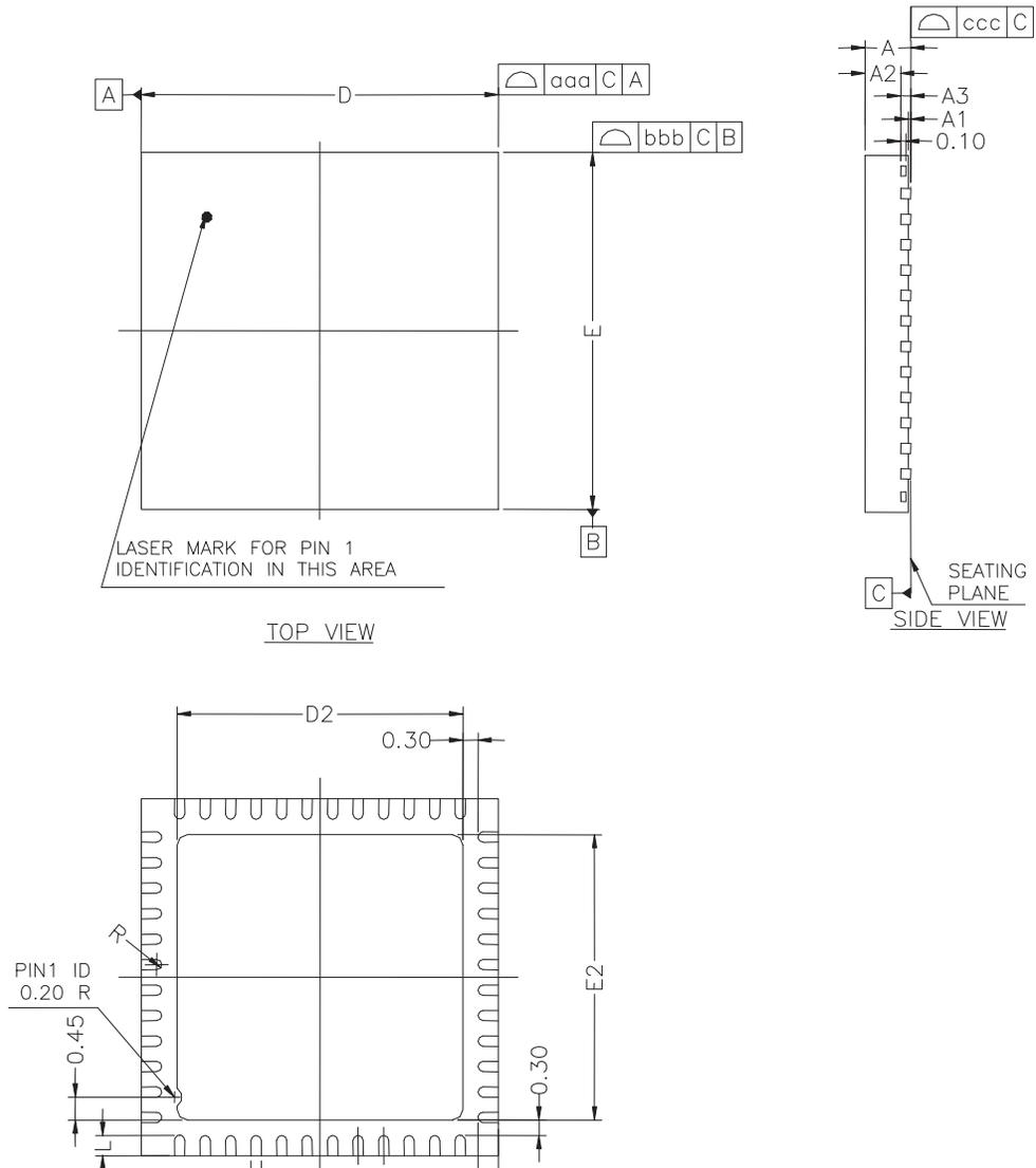
**Table 38-6.** 48-pad QFN Package Dimensions (in mm)
